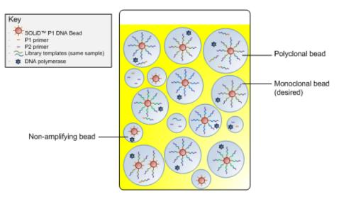
Figure 5 Emulsion after amplification (ePCR).
