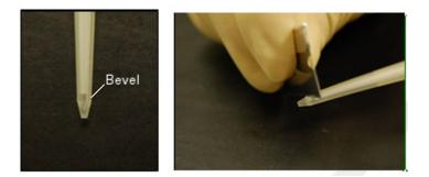
Figure 14 Cutting the Combitip Plus tip for emulsion dispersion.
