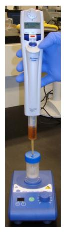
Figure 13 Correct placement of Combitip Plus into sample port in SOLiD™ ePCR Tube cap.
