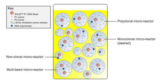
Figure 4 Emulsion before amplification (ePCR).
